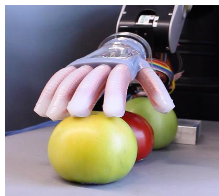
Fig 2: Hand-like pneumatic gripper
